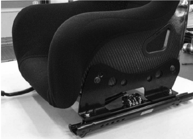
Seat rails and seat adapters fitted as previously in Cup
